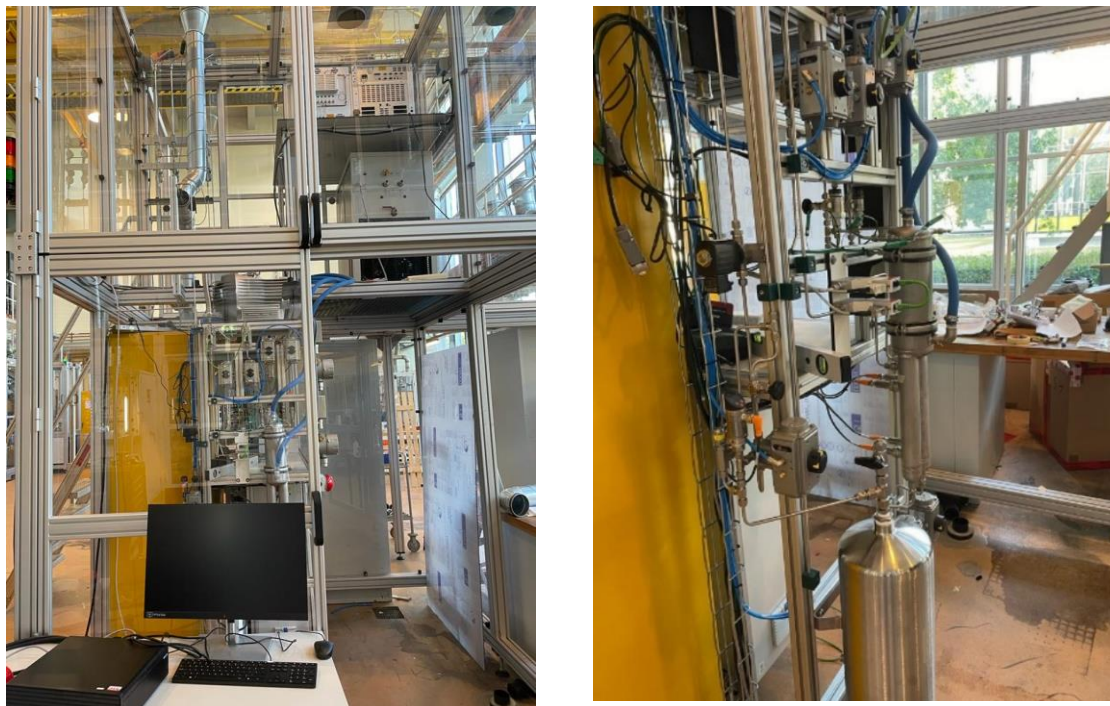
Operator desk, GC, chiller, vessels with level sensors
