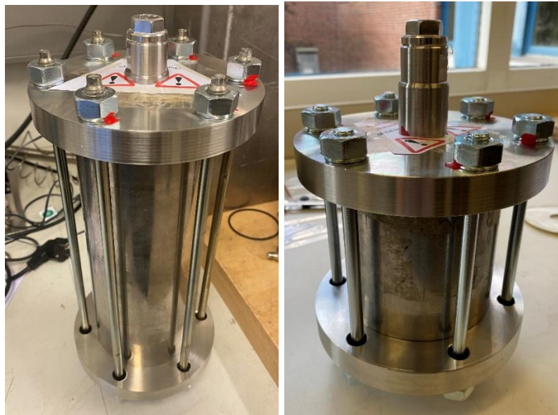
Figure 2. Demonstrator (left) and lab-scale (right) envelope-type membrane modules fabricated at the Institute of Membrane Research of Helmholtz-Zentrum Hereon with the prototype A multilayer TFCM.
