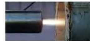
Figure 1 : plasma flame of a 2 MW torch
