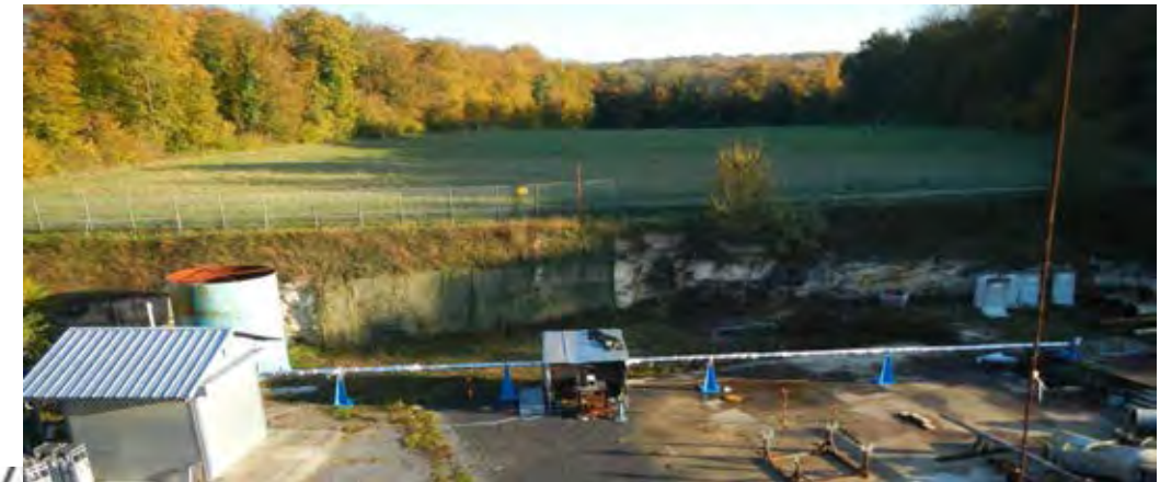
Medium-scale test pipeline 40 m long, 2" i.d. (INERIS)
