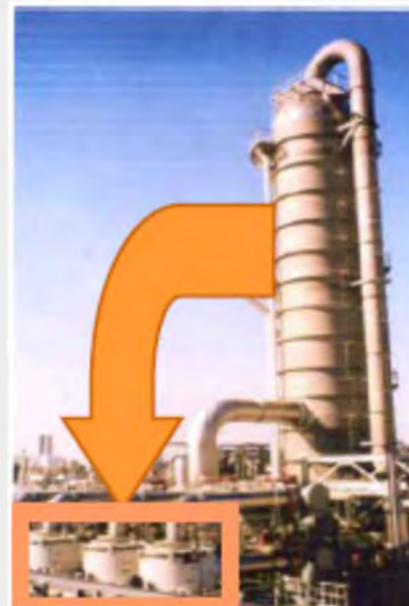
Conventional fixed bed reactor vs 40 times intensified reactor. (Source: Dow Chemical, proceso HOCl)
