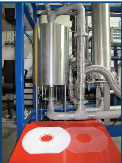
Thin-film composite (TFC) membrane fabrication: polymer → membrane → module
