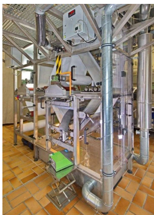
Pilot scale membrane coating facility for thin-film composite membranes (TFCM)
