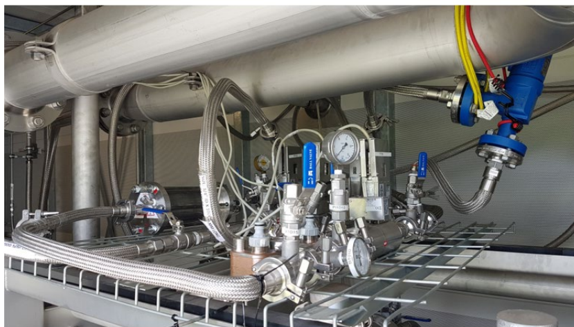
Figure 8: Hereon's installed membrane module tested at DMT premises
